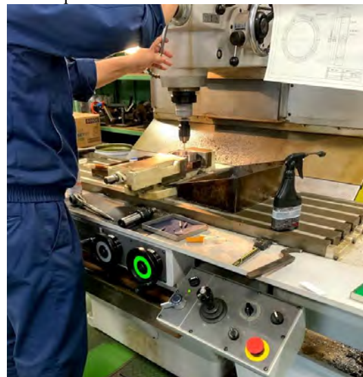
Figure 2 Processing using NC programming.
