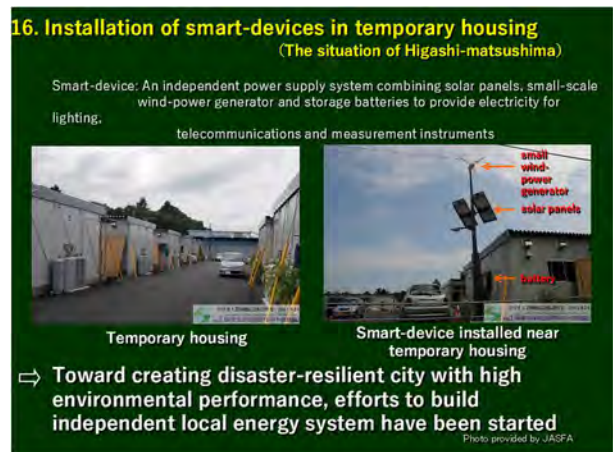
Figure 1 Self-sustaining lighting system in the area of temporary houses
