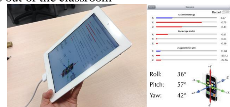
Figure 12: During a MDTE class demonstration, the iPad is tilted to a specific angle and based on the values of the accelerometer displayed on the app, the students are required to calculate and analyze the values based on the theoretical knowledge they have learned in class
