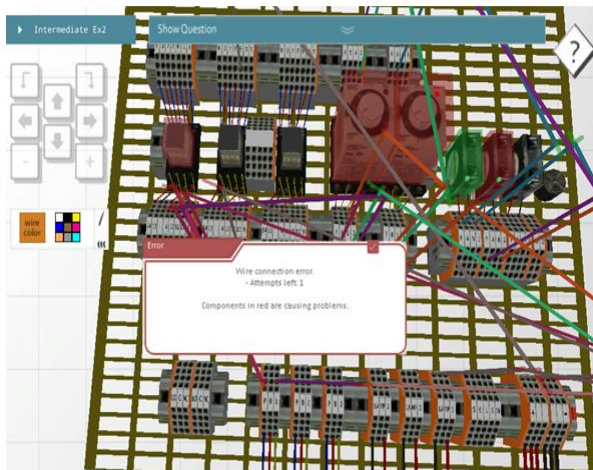
Figure 5 : Wrong Wiring submission
