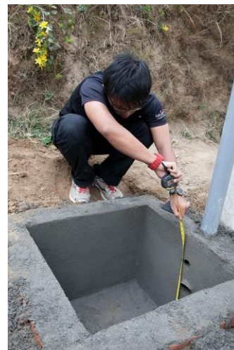
Figure 6. A student measuring the dimensions of the buffer tank upstream to the storage tank
