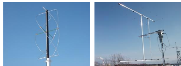
Figure 8 turn-style antenna and Yagi beam antenna
