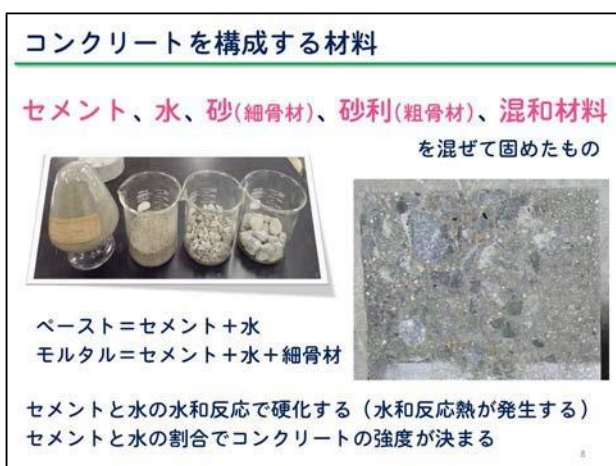
(a) materials of concrete
