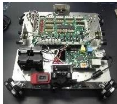
Figure 3 Basis robot (omnidirectional mobile robot)
